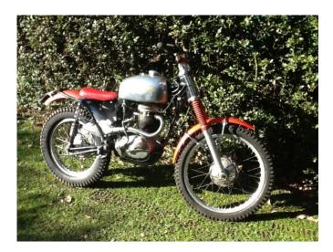
**BSA B40 350cc pre 65 trials bike**, nominally 1964, in the original Harry Foster 60/70's Otter oil in frame, slimline alloy tank, ali rims on cub hubs, GB Trials gearbox, MP style forks, red guards, black seat, engine sounds sweet with Boyer ignition. Inspection/test can be arranged.
